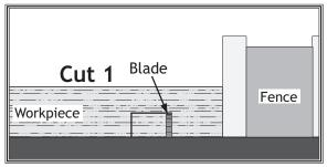
**Figure 52.** First cut when using a single blade for making a dado.
